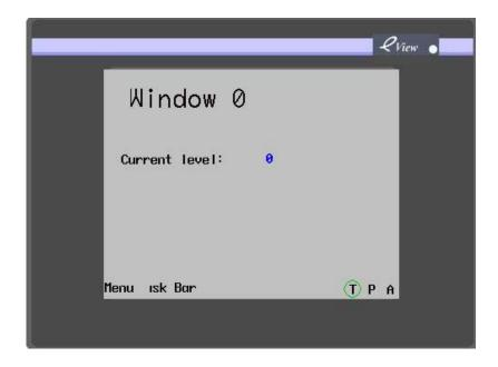
Because no password is entered, the current security level must be 0 when the project runs. Switch to window 4 and set the (**Security Level**) to (**Medium**, that is, 1) in the (**Window Properties**) window, as shown below:
