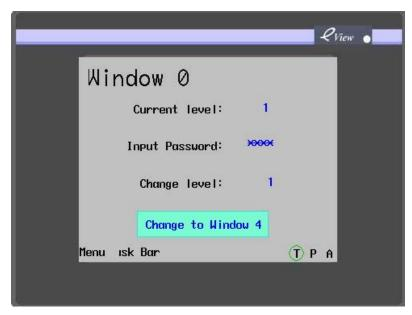
Press the function key, and the system changes to window 4. If the user enters the value 0 in the (**Change Level**) frame, the current security level changes to 0 immediately, and then, the system cannot switch to window 4, as shown in the figure below:
