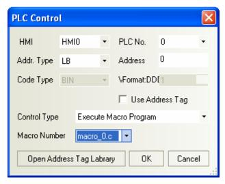
**eAddress Type/Address**: The address of the register triggering the execution of the macro instruction. If this bit is set to "1", the macro code will be executed; if it is set to "0", the macro instruction will not be executed.
