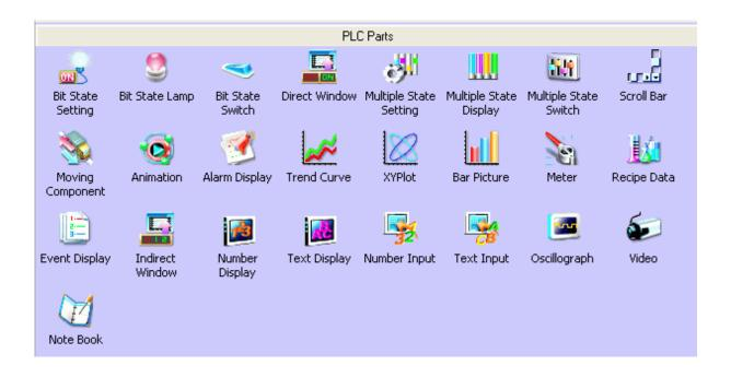
After creating a project and switch to the configuration screen edit window, you can drag parts to be used into the configuration window. For the detailed instruction for using the PLC parts, please refer to Chapter 6.
