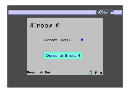
Press the function key, but the system fails to switch to window 4. The reason is that the current security level is 0, while that of window 4 is 1, so the user cannot access a window with higher security level from lower one. To access window 4, the user has to enter the password for the security level 1. The registers LW9040~LW9041 reserved by the system are used to enter passwords for different security levels. Add a numeric input component to window 0, as shown in the figure below:
