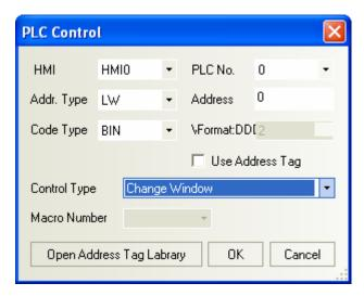
As shown in the above figure, we use LW0 to change window. Assume that the current window is Window 0. If LW0 changes to "4", the current screen will change to Window 4, and then the value "4" will be written back to register LW1.
