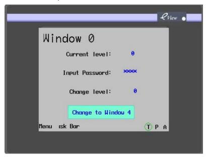
Enter 1 in the (**Change Level**) frame, but the current level will not change to 1 because it is not permitted to change a window with a lower security level to a window with a higher security level, as shown below:
