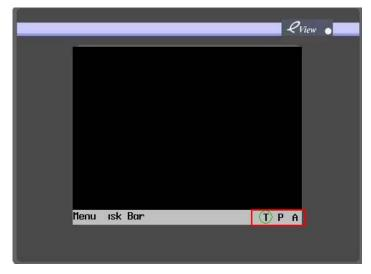
**Include fast selection window**: Determine whether to include the fast selection window. If this check box is selected, the user can use the parts in the fast selection window to switch over between different windows. If this check box is not selected, the fast selection window will not appear.
