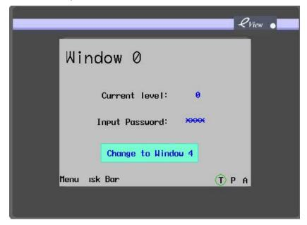
The current security level is 0, so the (**Change Window 4**) button is unavailable. Enter the password **1111**, and the current security level changes to 1, as shown in the figure below:
